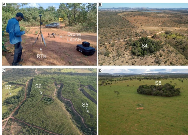
Figure 2. UAV survey and aerial views of dolines: (A) RTK-GPS and LiDAR system coupled to the drone; (B) overflight of sinkhole S4; (C) sinkholes S5–S7 under denser vegetation; (D) sinkhole S8 with dense vegetation.
